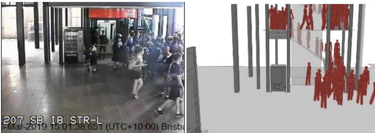
Figure 13 An example of a calibration and validation process (concourse level) – verify that at a specific time there is a correspondence between the footage and the microsimulation model.
