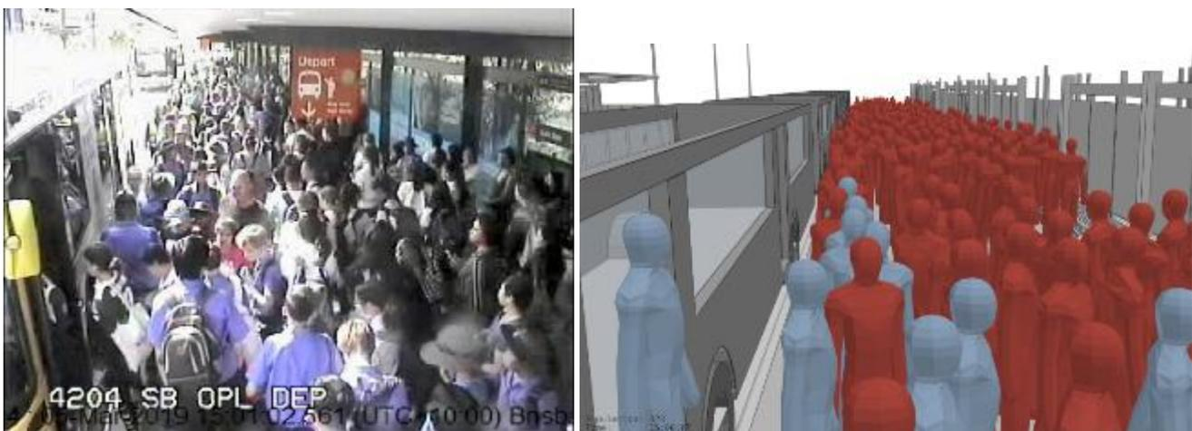
Figure 14 An example of a calibration and validation process (platform level) – verify that at a specific time there is a correspondence between the footage and the microsimulation model.
