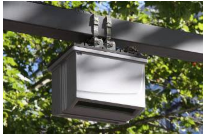
Figure 9 - Melbourne's pedestrian counting using overhead infrared sensors. Source: http://www.pedestrian.melbourne.vic.gov.au/
