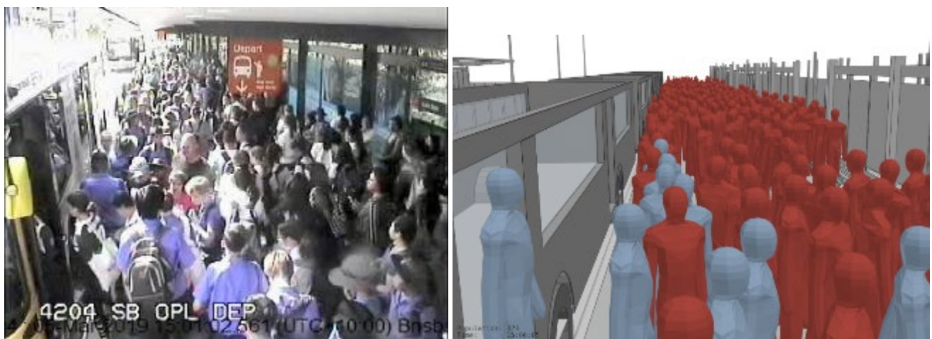
Figure 15 An example of a calibration and validation process (platform level) – verify that at a specific time there is a correspondence between the footage and the microsimulation model.
