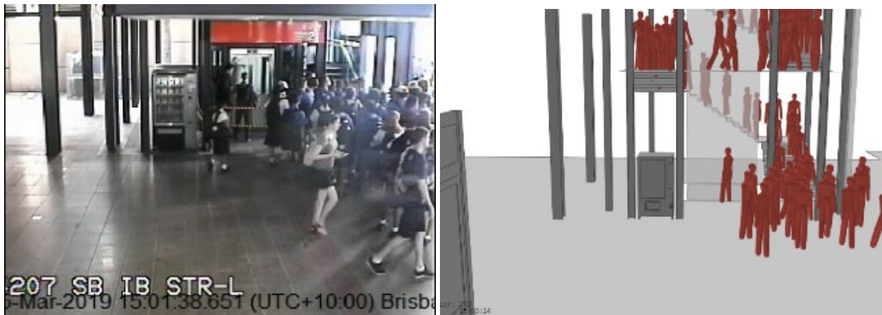
Figure 14 An example of a calibration and validation process (concourse level) – verify that at a specific time there is a correspondence between the footage and the microsimulation model.
