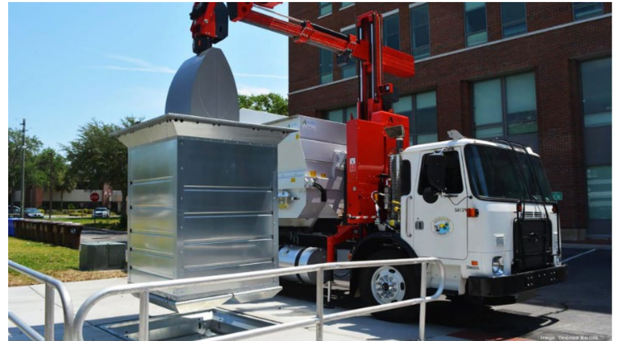
In Kissimmee, Florida, the first US city to install submerged containers, a standard collection truck modified with a hoist that can be used with both submerged and surface containers
