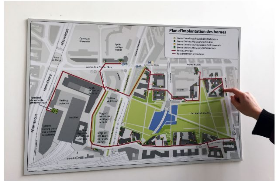
Compactor container fed by pneumatic tube; Map of pneumatic pipe network at Clichy-Batignolles (collection terminal is at far left)
