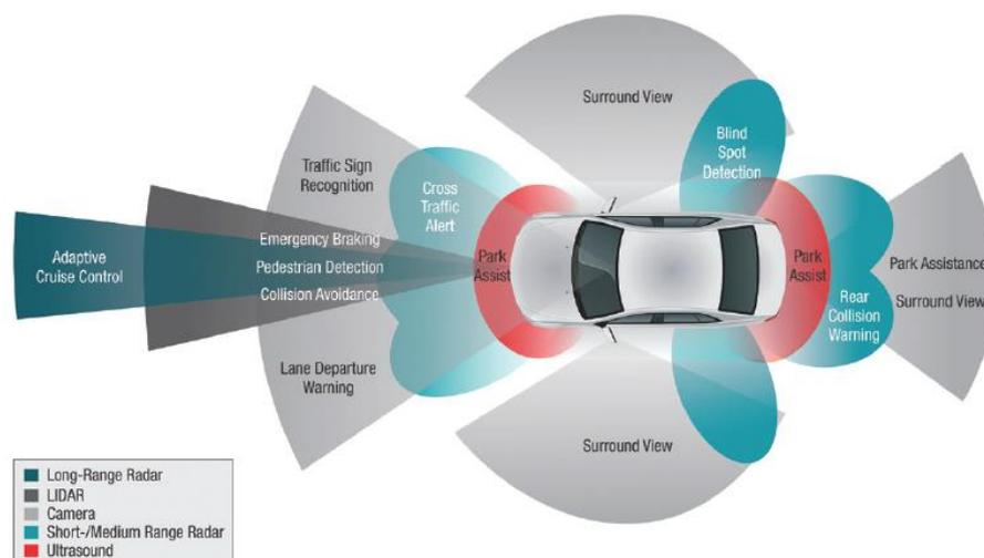
Figure 1: Typical AV sensor arrangement (Texas Instruments)
