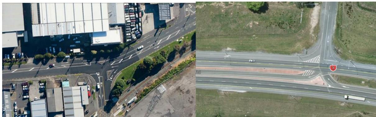
**Figure 6: Example of Painted and Raised Island Seagull Intersection**
