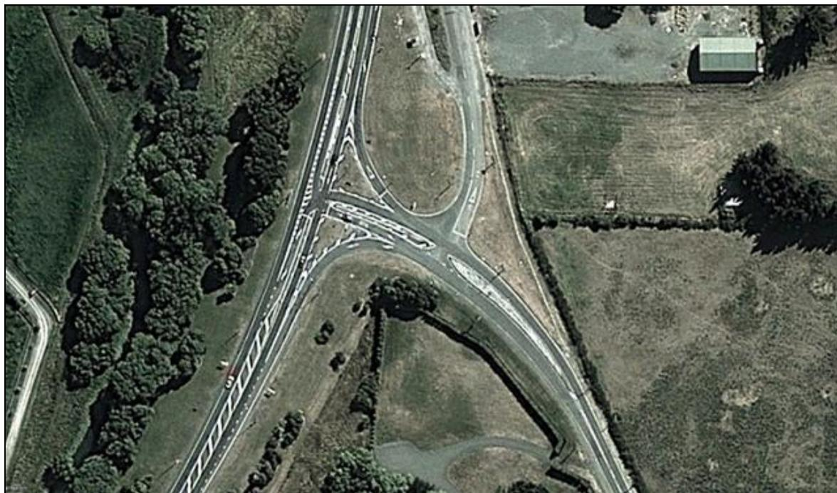
**Figure 1: Typical Seagull intersection (with LTSL) in New Zealand**
