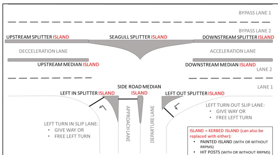
**Figure 7 – Seagull Layout Variable - Island Types**
