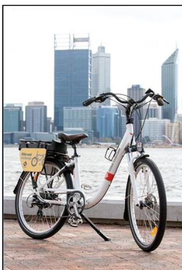
An eBike is a bicycle with an electric motor and rechargeable battery that provides assistance to the rider. There are currently two categories of eBikes in WA, those with a maximum power output of 200 watts and 'Pedalecs' which comply with *European Standard EN 15194* and have a maximum power output of 250 watts. In 2012, the Australian Government adopted the EU design standard and 250 watt pedalecs (which are the eBikes used for the trial) became legal in WA in April 2015.
